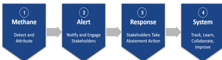
Figure: Four components of Methane Alert and Response System
